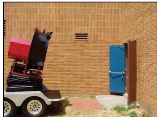
Other Fan positioned 12 ft from the doorway
