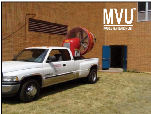
MVU™ positioned 21.5 ft from the doorway
